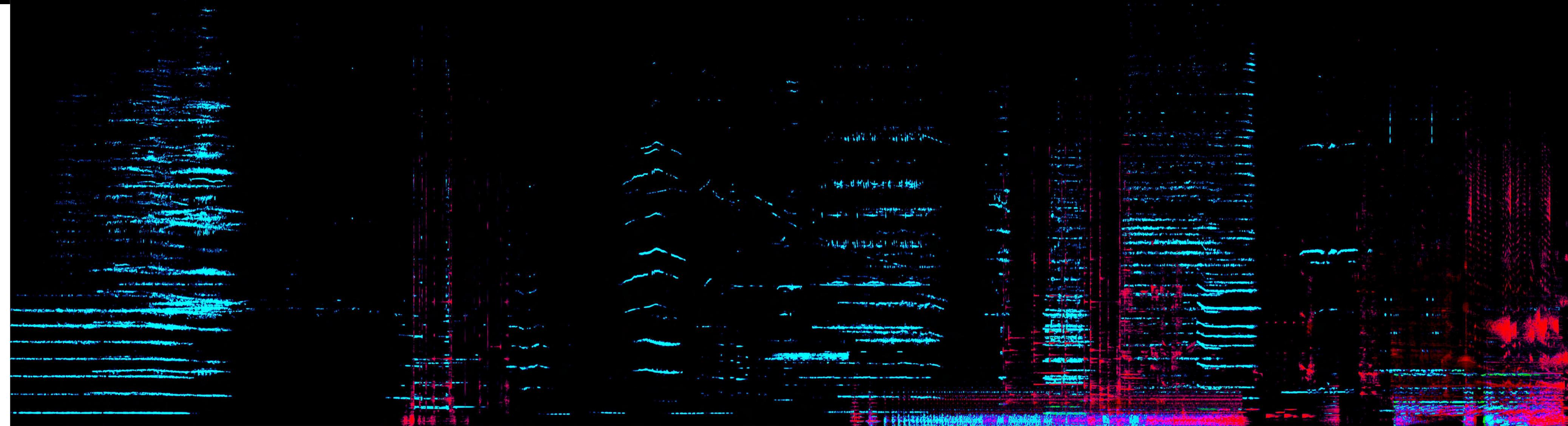
"As BPM increases beyond 10 Hz, rhythmic pulses generate overtones that gradually overlap, leading to the perception of continuous pitch, with full pitch recognition occurring around 1200 BPM (20 Hz)."
